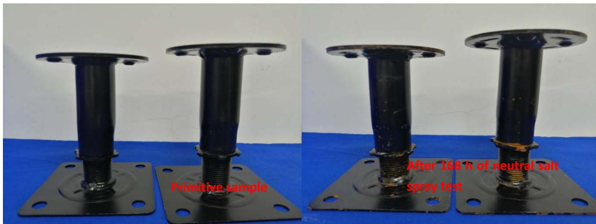
Figure5 Photos after test
